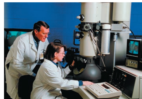
FIGURE 31.10 An electron microscope makes practical use of the wave nature of electrons. The wavelength of electron beams is typically thousands of times shorter than the wavelength of visible light, so the electron microscope is able to distinguish detail not visible with optical microscopes.
