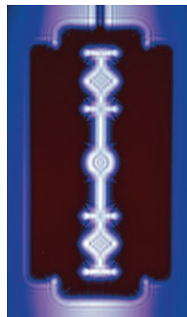
FIGURE 29.10 Diffraction fringes are evident in the shadows of monochromatic (single-frequency) laser light. These fringes would be filled in by multitudes of other fringes if the source were white light.
