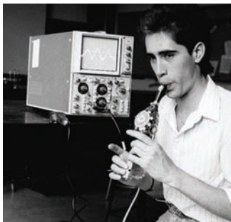
FIGURE 21.4 James displays a sound signal on an oscilloscope.
