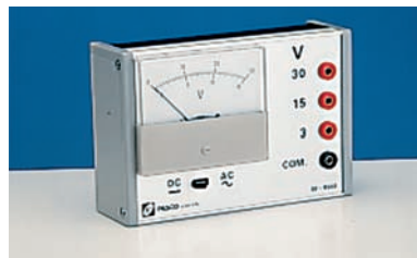
FIGURE 24.18 Both the ammeter and the voltmeter are basically galvanometers. (The electrical resistance of the instrument is made to be very low for the ammeter and very high for the voltmeter.)
