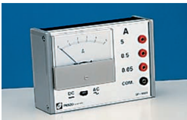
FIGURE 24.18 Both the ammeter and the voltmeter are basically galvanometers. (The electrical resistance of the instrument is made to be very low for the ammeter and very high for the voltmeter.)
