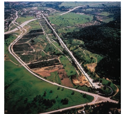
FIGURE 35.25 The Stanford Linear Accelerator is 3.2 km (2 mi) long. But to electrons moving through it at 0.9999999995c, the accelerator is only 3.2 cm long. The electrons start their journey in the foreground and they smash into targets, or are otherwise studied, in the experimental areas beyond the freeway (near the top of the photo).
